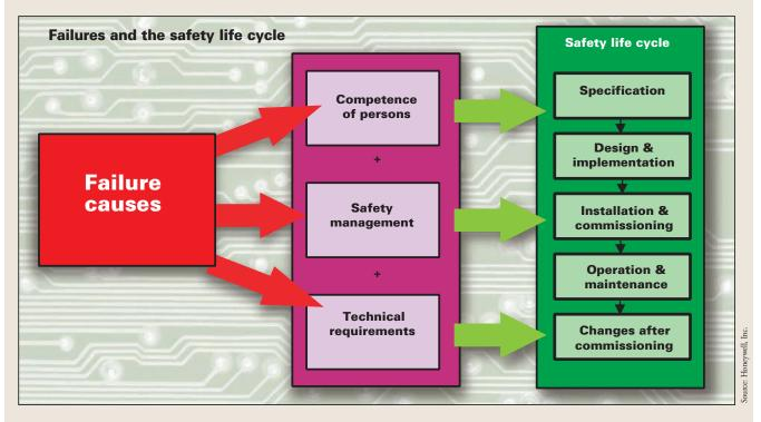
Safety concerns mentioned in ANSI/ISA-S84.01-1996 and IEC 61508 safety standards, and typically referenced in the safety life cycle, find solutions through digital communications. The life-cycle model takes a whole view of plant safety and allows a broader appreciation of how to improve the safety of the entire plant.
