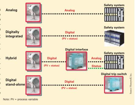
instrument at a 500-millisecond to 2-second rate. Because diagnostic status does not synchronize to the process measurement's output signal, safety interlocks must act on the analog 4–20 mA signal.
